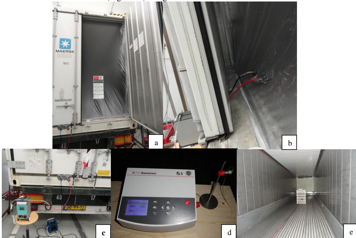
Figure 3, air tightness test of the CA container. Door opening closed with CA curtain [a], CO 2 injection tube going through the CA curtain [b], CO 2 concentration measurement from outside the container [c], CO 2 concentration sensor and recorder – PBI Dansensor CheckMate II [d], position of CO 2 injection tube outlet and CO 2 sensor inside the container [e].
