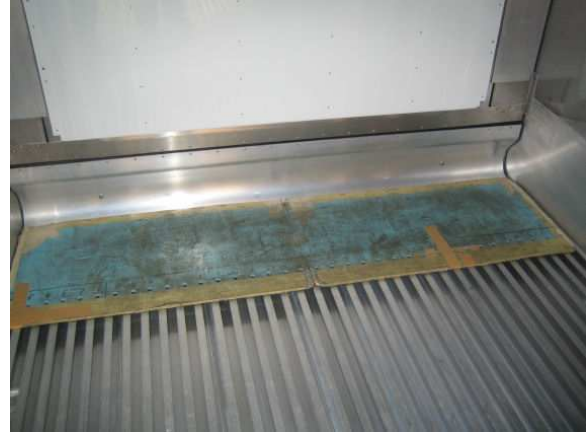
Figure 13: plating covering first 50 cm of T-bar for air circulation measurement (step 7 above).
