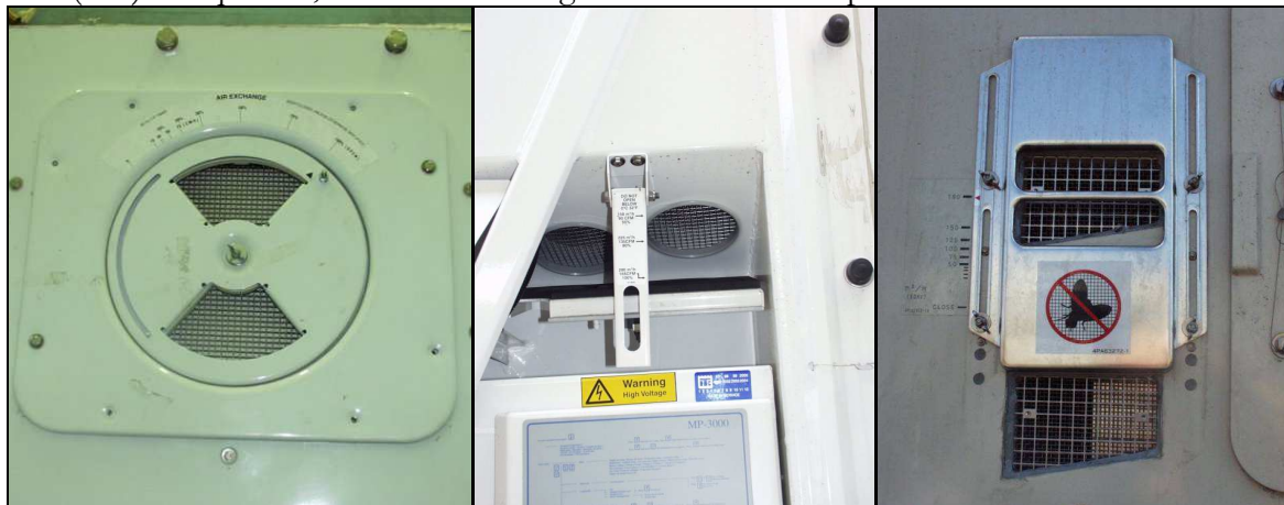
Figure 15: some of the most common fresh air vents (from left to right Carrier, Thermo King and Daikin).
